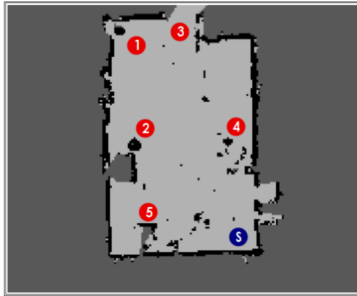
Figure 4. Map of testing process for the robot's navigation system. Red circles indicate predefined goal points, blue circle indicates start point.
